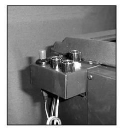
**Figure 8.25** Insert the rheostat control into its opening from beneath the control panel. Fit the rheostat nut on top and tighten the nut using an 11/16 in. wrench. Attach the black knob.
